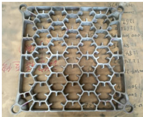
Lost Wax 3D printing (patternless)
